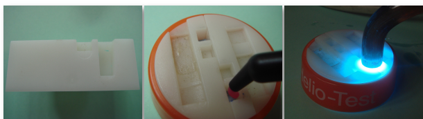
Figure 2 & 3– Sample's production in a Jig, 5mm deep
