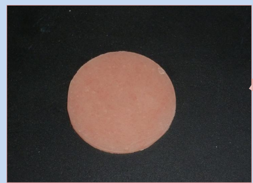
Resin disk-shaped specimens 50 x 2 mm
